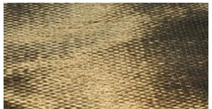
Fig 1. Basalt Fibre
